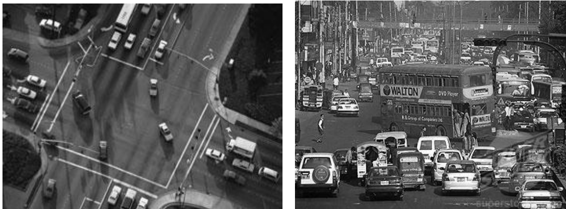
Figure 1: Traffic Movement at Signalized Intersection: Lane Based (Left) and Non-Lane Based (Right)
